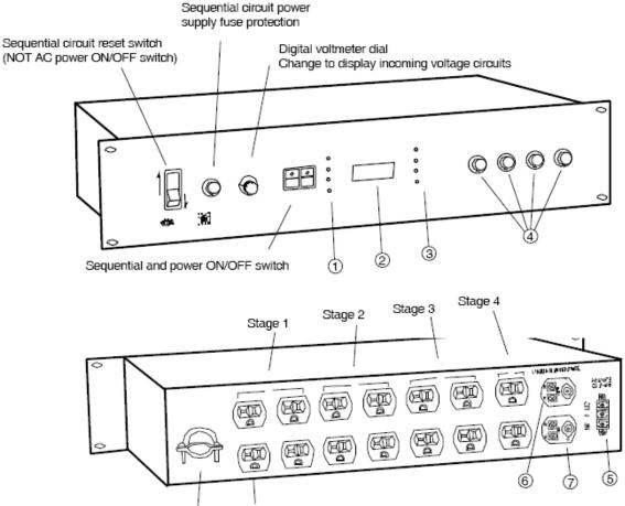
Romex connector for power hook-up 20-amp dual Edison U-grounded outlets
